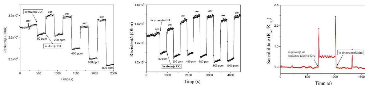
CO response/recovery of the sample with 5 layers (left) and 9 layers (middle), at 260 °C and titanate based nanotube's sensitivity to humidity (right), all samples on Al<sub>2</sub>O<sub>3</sub> transducers
