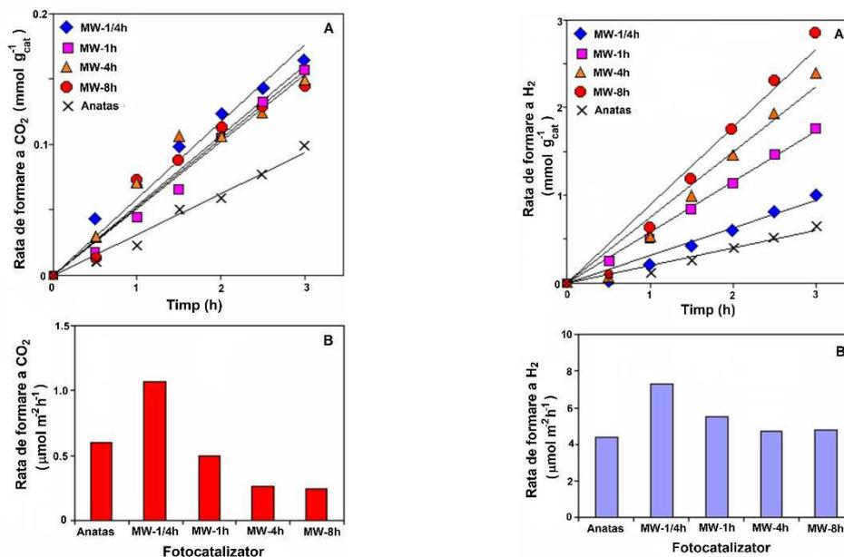
Photocatalytic test results: CO<sub>2</sub> (left) and H<sub>2</sub> (right), release by time, normalized to photocatalytic amounts (A) and corresponding reaction rate, calculated to surface unit (B)
