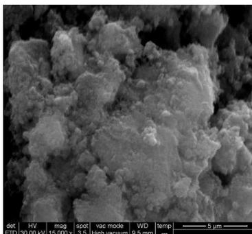
*SEM micrographs of the titanate based nanotubes sample, functionalized with biomaterial*
