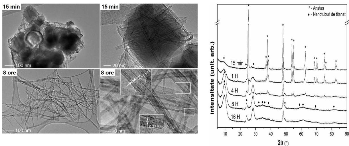
*TEM micrographs (left and middle, different magnifications) and X-ray diffractograms (right) of titanate based nanotubes, prepared by microwave assisted hydrothermal method*
