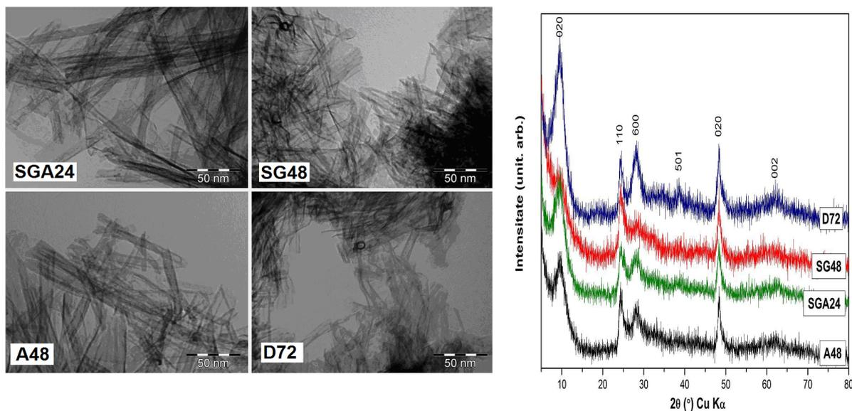
*TEM micrographs (left) and X-ray diffractograms (right) of titanate based nanotubes, prepared by conventional hydrothermal method*
