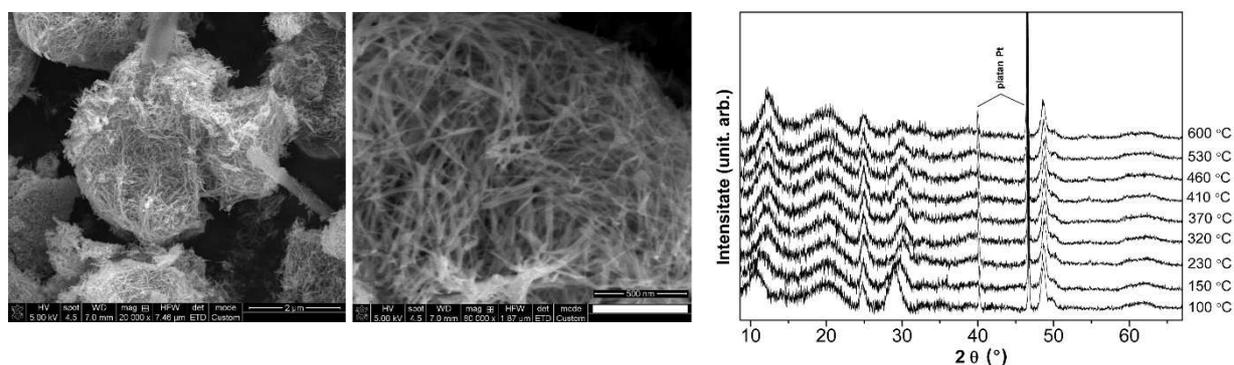
*SEM micrographs (left and middle) and in-situ X-ray diffractograms (right) of titanate based nanotubes, prepared by microwave assisted hydrothermal method*
