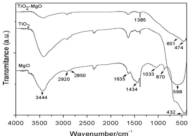
Fig. 4. FT-IR spectra of the heat treated oxides: TiO<sub>2</sub>, MgO, MgO-TiO<sub>2</sub>
