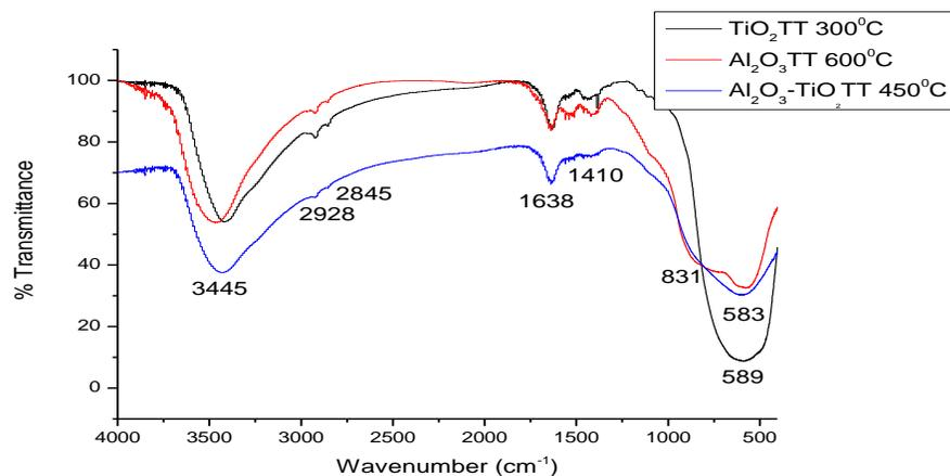
Fig. 5. FT-IR spectra of monocomponent and binary samples, thermally treated ( $\text{TiO}_2$ ,  $\text{Al}_2\text{O}_3$  and  $\text{Al}_2\text{O}_3\text{-TiO}_2$ )
