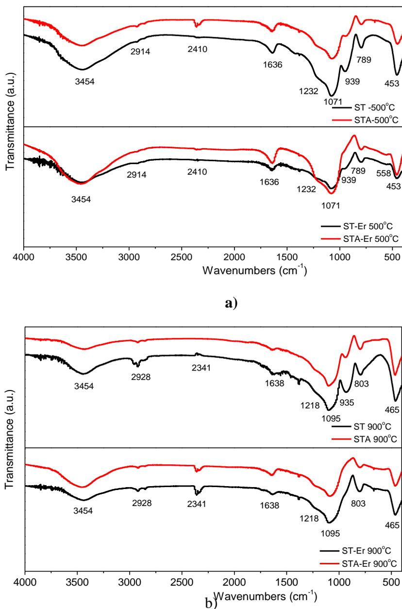
Fig.2. FT-IR spectra of thermally treated powders a) at 500°C and b) at 900°C
