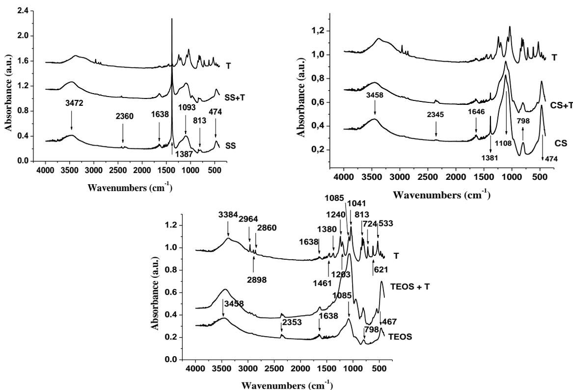
Fig.10. IR spectra of trichlorfon, pesticide-silica sol-gel composites and corresponding silica matrices obtained from various precursors, TEOS, CS and SS
