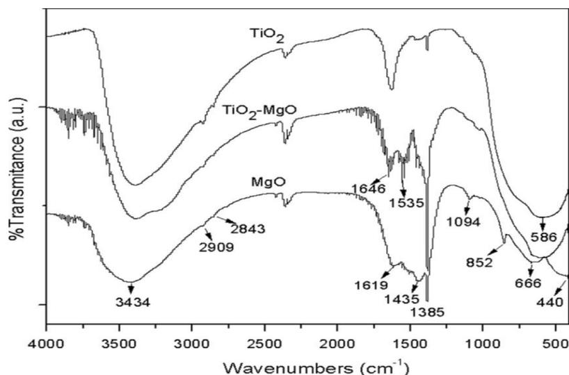
Fig. 3. FT-IR spectra of oxide powders obtained from synthesis: TiO<sub>2</sub>, MgO, MgO-TiO<sub>2</sub>
