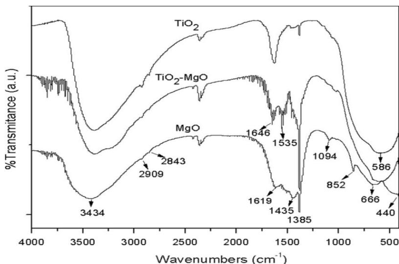
Fig. 3. FT-IR spectra of oxide powders obtained from synthesis:  $\text{TiO}_2$ ,  $\text{MgO}$ ,  $\text{MgO-TiO}_2$
