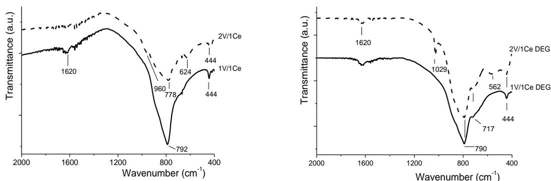
Fig.9. IR spectra of thermally treated samples (s) without DEG, (b) with DEG
