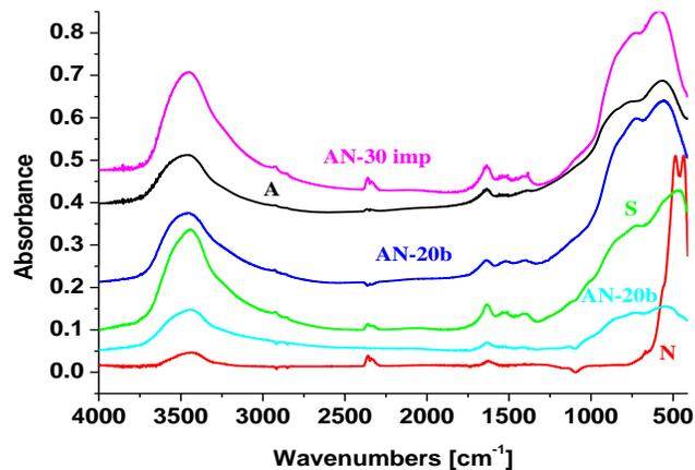
Fig. 7. The FT-IR spectra of samples A ( $\text{Al}_2\text{O}_3$ ), S ( $\text{NiAl}_2\text{O}_4$ ), AN20 (a and b) ( $\text{NiO}$ ), and AN30-imp sample ( $\text{Al}_2\text{O}_3$  doped with 30% Ni by method b)
