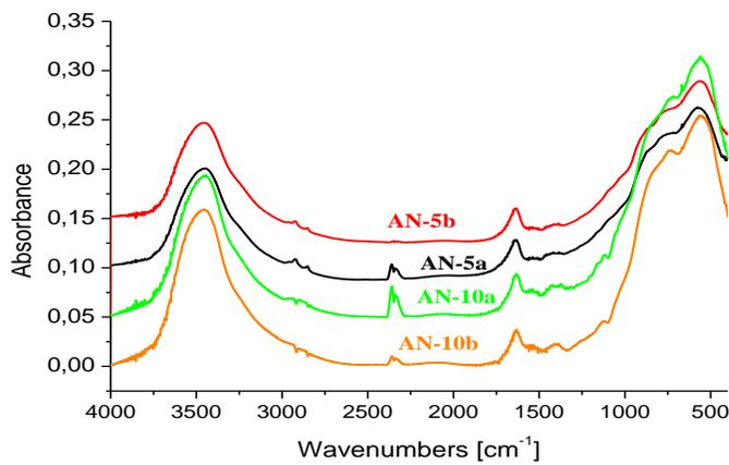
Fig. 6. The FT-IR spectra of alumina samples with 5% Ni (AN 5) and 10% Ni (AN 10)
