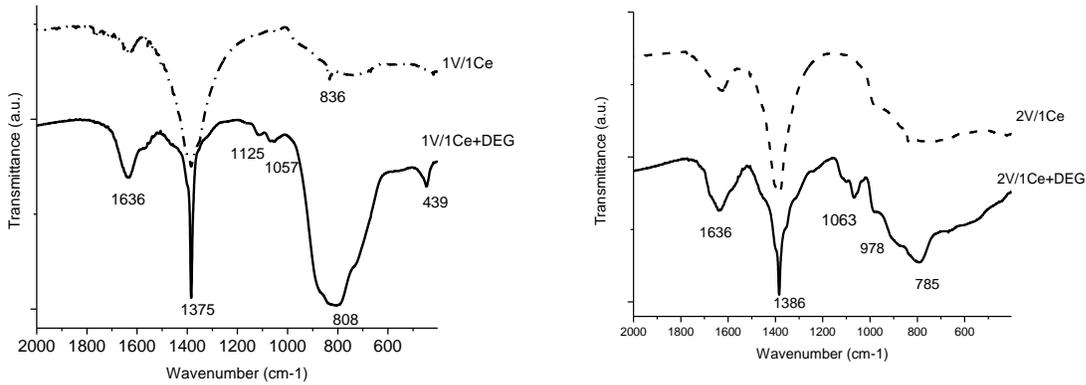
Fig. 8. The FT-IR spectra of the binary powders obtained from the synthesis: a) 1V/1Ce and b) 2V/1Ce with and without DEG
