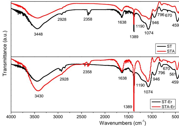
Fig.1. FT-IR spectra of as-synthesis gels
