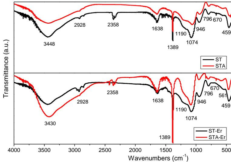
Fig.1. FT-IR spectra of as-synthesis gels
