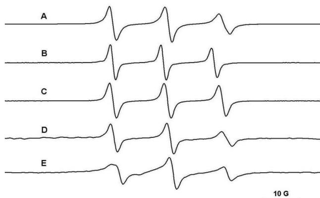
**Figure 20.** The EPR spectra of TEMPO (A), L62NO (B), P123NO (C), PEG8000-NO (D) and F127NO (E) spin probes encapsulated in PPG2000 /  $\alpha$ -CD gel, in DMF.
