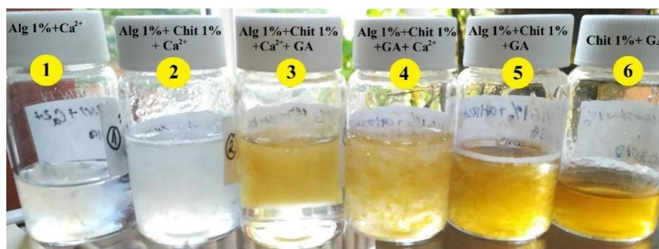
**Figure 12.** Gel samples 1) Alginate +  $\text{Ca}^{2+}$ , 2) Alginate + Chitosan +  $\text{Ca}^{2+}$ , 3) Alginate + Chitosan +  $\text{Ca}^{2+}$  + glutaraldehyde, 4) Alginate + Chitosan + glutaraldehyde +  $\text{Ca}^{2+}$ , 5) Alginate + Chitosan + glutaraldehyde, 6) Chitosan + glutaraldehyde.
