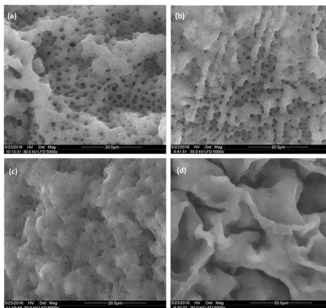
**Figure 2.** Morphology images of the surface of xerogels: Alg (a), Alg-Ad (b), Alg-1,3- $\beta$ -CD (c) and Alg-1,3- $\beta$ -CD / Alg-Ad (d).
