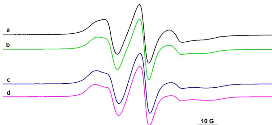
**Figure 11.** The EPR spectra of spin-labeled alginate gels in the absence or presence of AuNPs: a) Alg-T, b) Alg-T / AuNP, c) Alg-1,2- $\beta$ -CD-T, d) Alg -1,2- $\beta$ -CD-T / AuNP.
