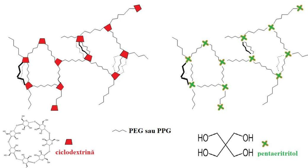
**Figure 16.** Schematic representation of polymer gel networks consisting of cyclodextrin or pentaerythritol with PEG or PPG, adapted after [18].
