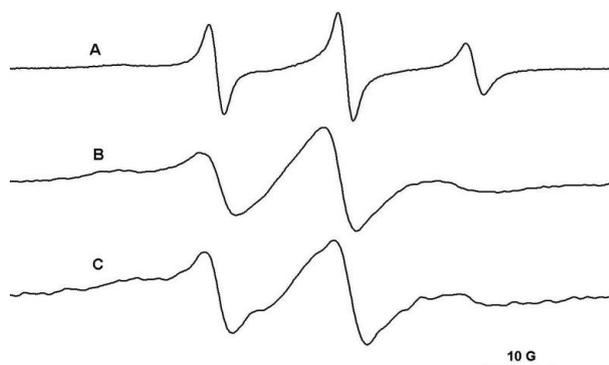
**Figure 18.** The EPR spectra of TEMPO (A), L62NO (B) and P123NO (C) spin probes encapsulated in PPG2000 /  $\alpha$ -CD gel, in water.
