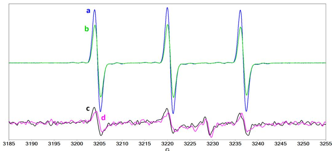
**Figure 30.** The EPR spectra of CPH adducts formed by UVA irradiation of a solution containing riboflavin and a) collagen, b) collagen + SOD, c) collagen + HA and d) collagen + HA + SOD.
