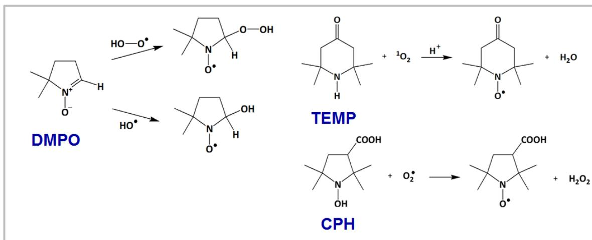
**Figure 26.** The structures of the spin traps used [32].
