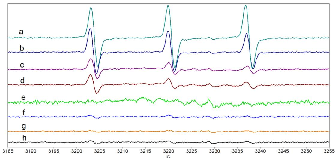
**Figure 31.** The EPR spectra of TEMPONE formed after UVA irradiation of systems: a) H<sub>2</sub>O, b) collagen + riboflavin, c) collagen, d) PESCHKE solution, e) tears, f) collagen + HA, g) collagen + HA + HSA + LF, h) HSA + LF + LYZ.
