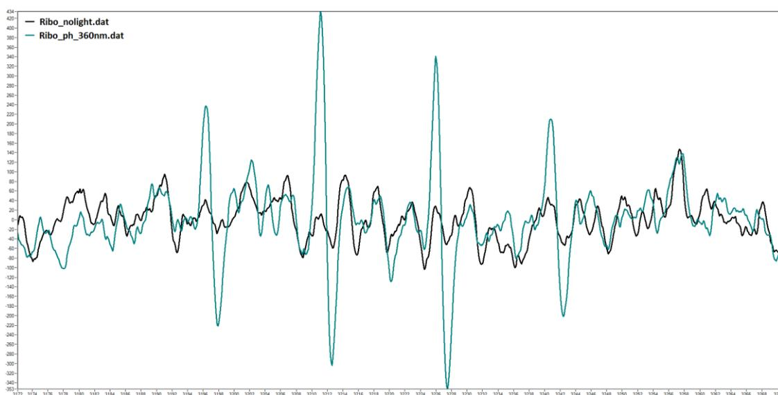
**Figure 27.** The EPR spectrum of riboflavin / DMPO solution in the absence (black) and in the presence of light (cyan).
