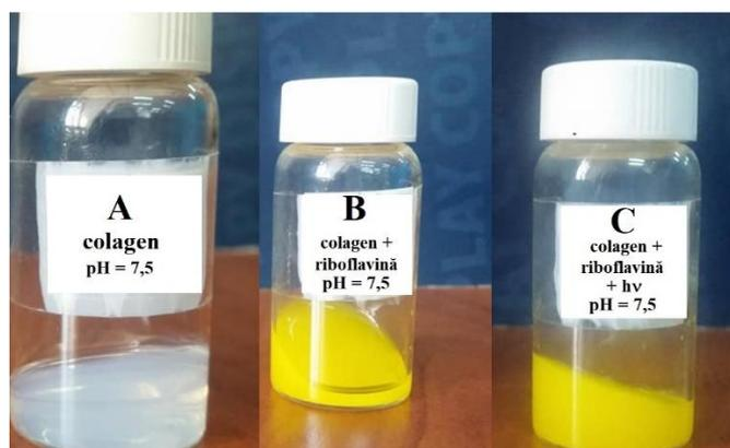
**Figure 24.** Collagen gels formed at pH = 7.5 in the absence of riboflavin (A), in the presence of riboflavin before exposure to UVA radiation (B) and after exposure to UVA radiation (C).
