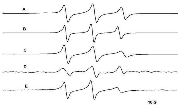
**Figure 19.** The EPR spectra of TEMPO (A), L62NO (B), P123NO (C), PEG8000-NO (D) and F127NO (E) spin probes encapsulated in PPG2000 /  $\alpha$ -CD gel, in DCM.
