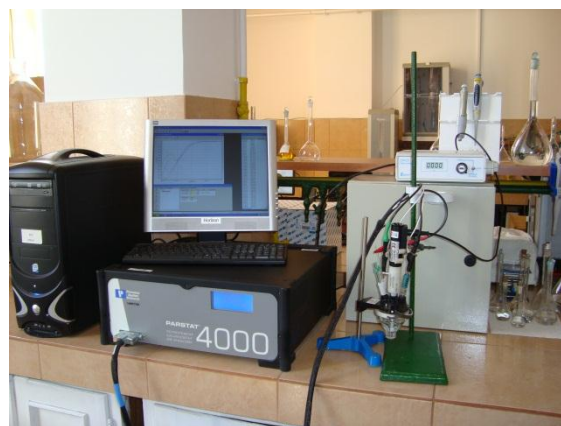
Potentiostat/galvanostat PARSTAT 4000 with Rotating Disk Electrode
